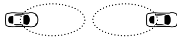
Figure 4. Each vehicle in a platoon is equipped with directional communication capabilities, selectively increasing gain to the front or to the back, e.g., by exploiting beamforming. This allows a vehicle to exploit the antenna gain for both transmission and reception.
