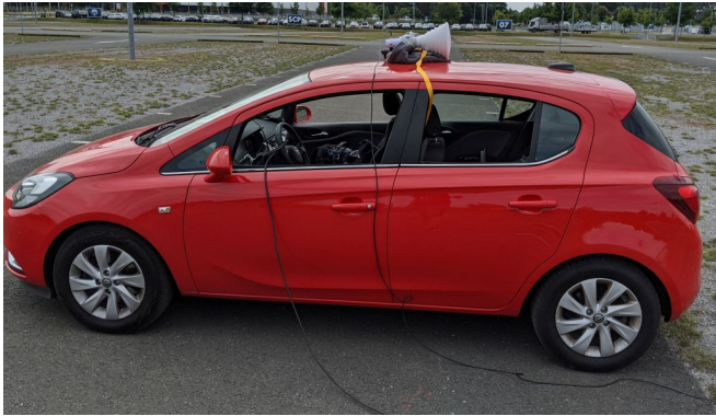
Figure 3. Antenna with (physical) directionality characteristics serving as an ideal model of (electrical) beamforming.
